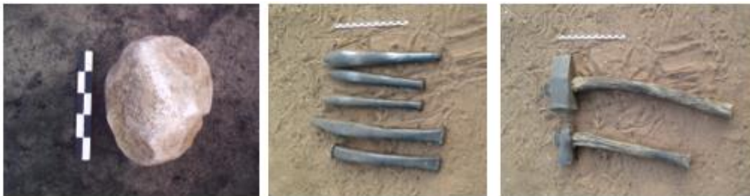
Figure 4: hammers (one stone hammer, five local iron hammers without handles and two modern hammers with wooden handles)
